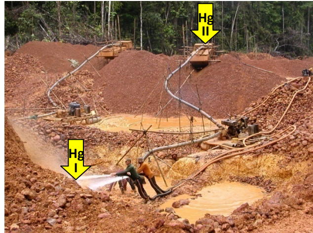
Figure 6. Application of mercury in different stages of the small-scale gold mining process
